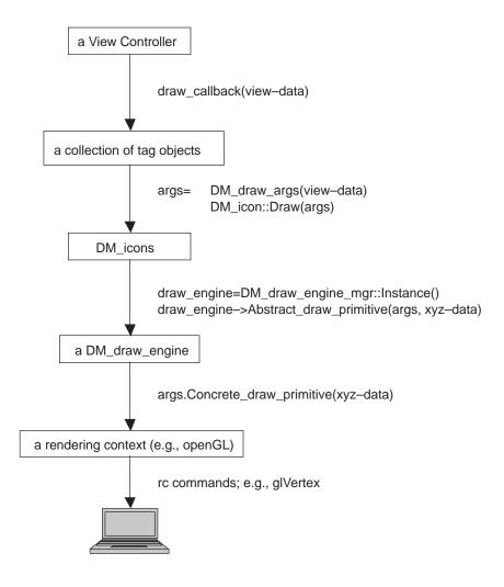
Figure 2-1. Draw Command Pipeline
