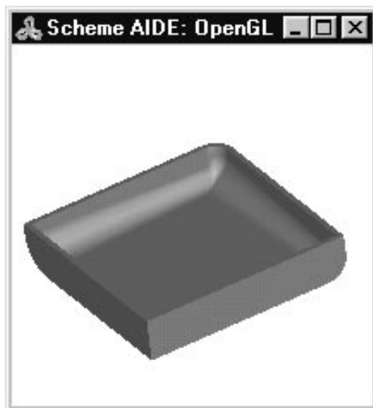
Figure 6-7. Shelling with tolerant modeling is faster
