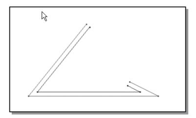
The issue arrives when offsetting a greater amount leaves segments that do not intersect outside of the inserted gap edges.
